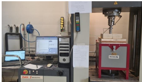
Fig. 9.1 – Customized swelling setup assembled on the Zwick machine. The setup is assembled inside the oven and the shaft connected to the load cell. A thermocouple is placed in the water bath.
