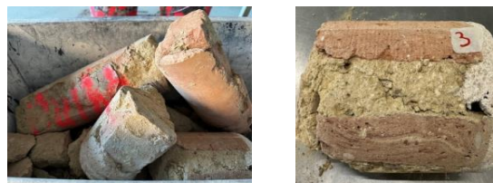
Fig 7.1 - Drilled core from an old masonry in Austria.
